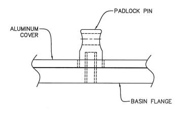
DETAILD SIDE VIEW OF PADLOCK PIN INSTALED
