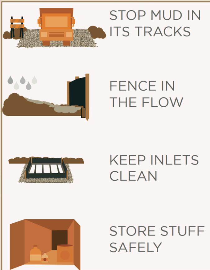
Sediment can block drains and contaminate stormwater. To prevent this, install and maintain a pad at the construction entrance to ensure that vehicles do not carry mud and dirt onto the roads.
